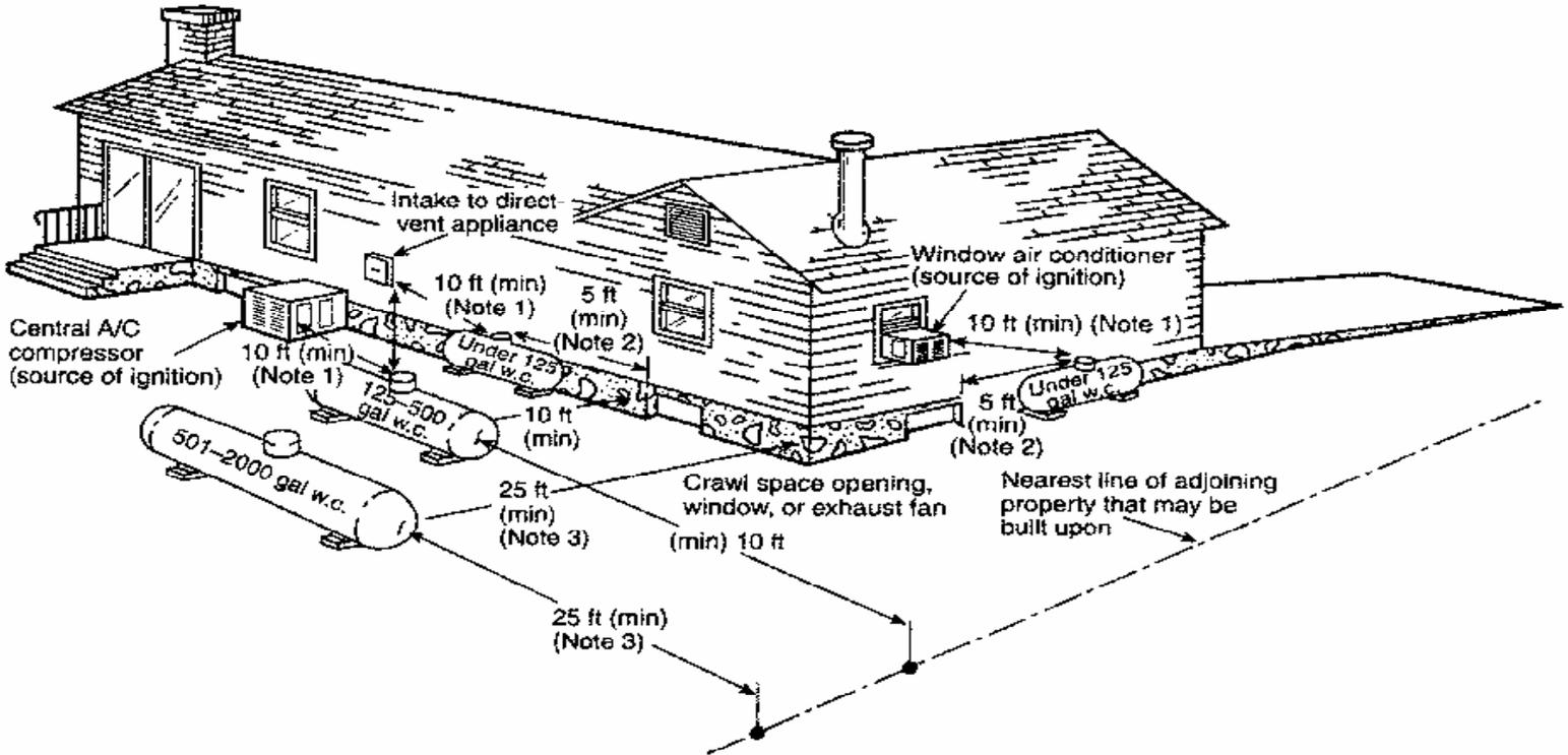
Note 1: Regardless of its size, any ASME container filled on site must be located so that the filling connection and fixed maximum liquid level gauge are at least 10 ft from any external source of ignition (such as open flames, window A/C, and compressors), intake to a direct-vented gas appliance, or intake to a mechanical ventilation system.
